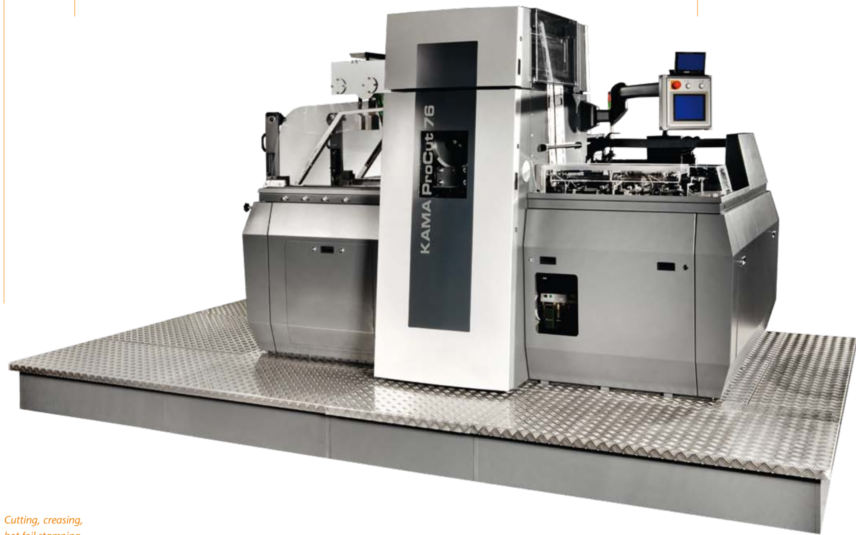
The compact main drive with worm gear ensures smooth running. Low maintenance.
